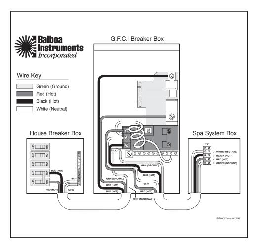
\* Actual wiring of GFCI will vary by manufacturer of GFCI. The GFCI shown is a Square D. Improper wiring of GFCI may result in permanent damage to spa system box. Repair / replacement of spa system box is not covered under warranty when damage results from improper wiring.
