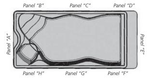
**NOTE:** Note: The above drawing illustrates the panel placement on the swim spa. **WARNING:** Do Not Remove Access Panels Without Turning Off Power To The Swim Spa.
