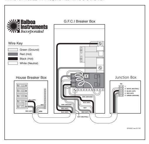
\* Actual wiring of GFCI will vary by manufacturer of GFCI. The GFCI shown is a Square D. Improper wiring of GFCI may result in permanent damage to swim spa system box. Repair / replacement of swim spa system box is not covered under warranty when damage results from improper wiring.
