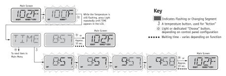
NOTE: If power is interrupted to the system, Time-of-Day will need to be reset.
