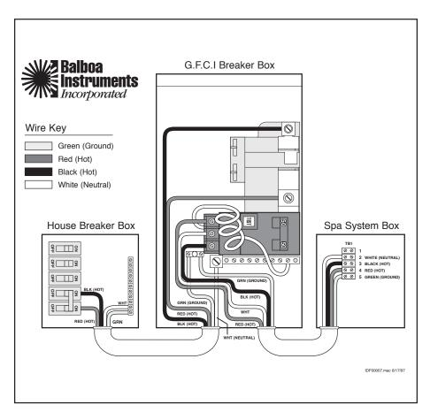
\* Actual wiring of GFCI will vary by manufacturer of GFCI. The GFCI shown is a Square D. Improper wiring of GFCI may result in permanent damage to spa system box. Repair / replacement of spa system box is not covered under warranty when damage results from improper wiring.
