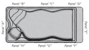
**NOTE:** Note: The above drawing illustrates the panel placement on the swim spa. **WARNING:** Do Not Remove Access Panels Without Turning Off Power To The Swim Spa.
