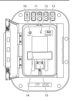
Select Button: Press to toggle between: bass, treble, balance, fader, equalizer, area, loudness and local/distance settings.
