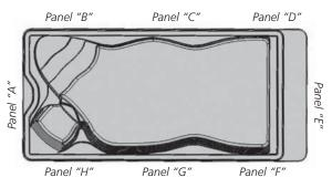
**NOTE:** Note: The above drawing illustrates the panel placement on the swim spa. **WARNING:** Do Not Remove Access Panels Without Turning Off Power To The Swim Spa.
