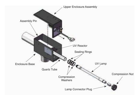
Figure 2: Mast3rPur System Exploded View
