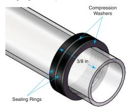
Figure 3: Quartz Tube Seal Assembly Detail
