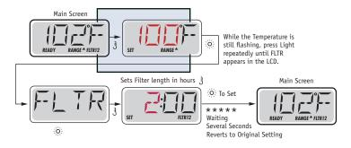
If Filter Cycle 2 is enabled, Filter 12 will appear in the LCD. If Filter is disabled, Filter 1 will appear.
