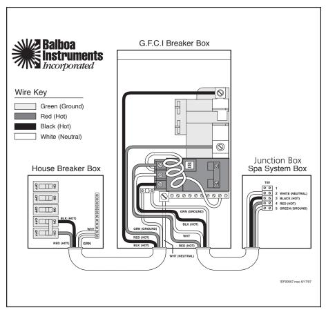
\* Actual wiring of GFCI will vary by manufacturer of GFCI. The GFCI shown is a Square D. Improper wiring of GFCI may result in permanent damage to swim spa system box. Repair / replacement of swim spa system box is not covered under warranty when damage results from improper wiring. Actual wire attachment points on the junction box may vary with different models. Always refer to the wiring diagram inside the junction box for proper connection.
