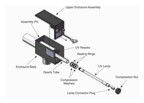
Figure 2: Mast3rPur System Exploded View
