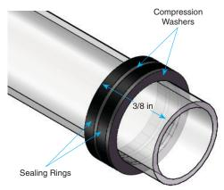
Figure 3: Quartz Tube Seal Assembly Detail
