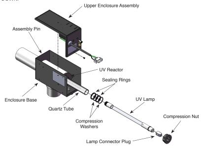
Figure 2: Mast3rPur System Exploded View
