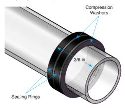
Figure 3: Quartz Tube Seal Assembly Detail
