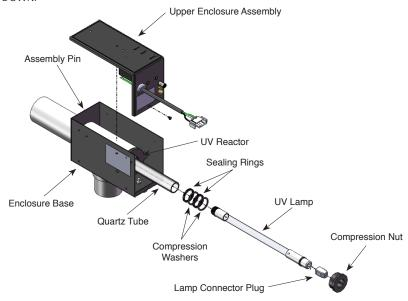
Figure 2: Mast3rPur System Exploded View
