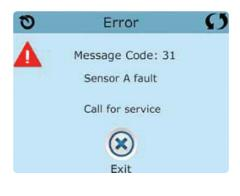
SENSOR A FAULT, SENOR B FAULT – SENSOR A: M031\*\*, SENSOR B: M032\*\* A temperature sensor or sensor circuit has failed. Call for Service.
